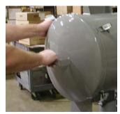
2. Remove the wing nut and the lid. Replace the filter element with the same size/brand.
