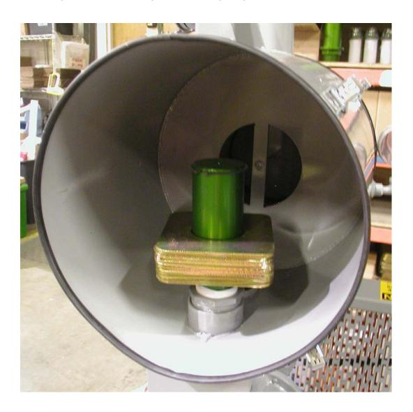
6. Install the provided snap ring into the groove at the top of the bonnet. If you don't have a tool as shown in the picture, you can use a needle nose pliers or similar.
