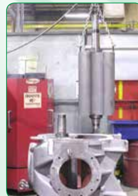
After a thorough inspection, the technician will clean, repair, test, and then paint the blower before returning it to the customer with a full one year warranty.
