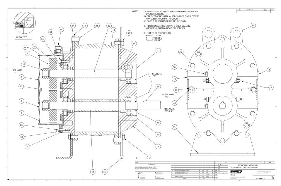
Assembly of UNIVERSAL RAI-G Series Gas Blowers, 3-1/2" through 5" Gear Diameter
