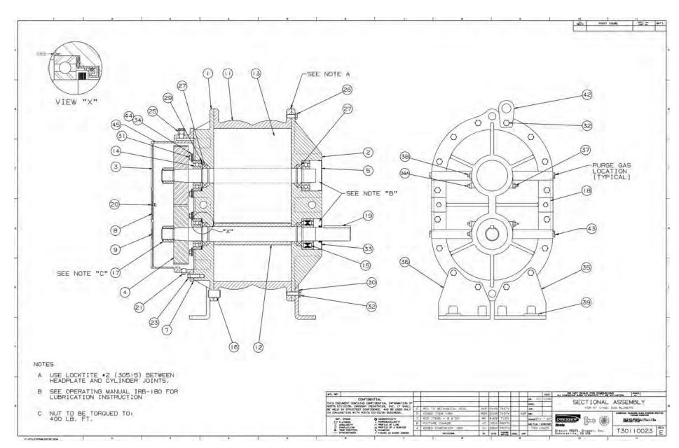
Assembly of UNIVERSAL RAI Series Gas Blowers, 6" Gear Diameter
