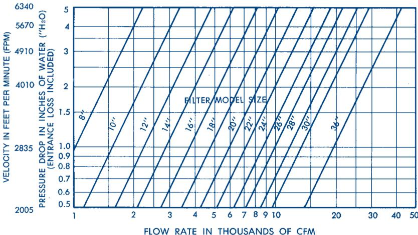
**Figure 2.** PRESSURE DROP FOR FILTER ELEMENTS
